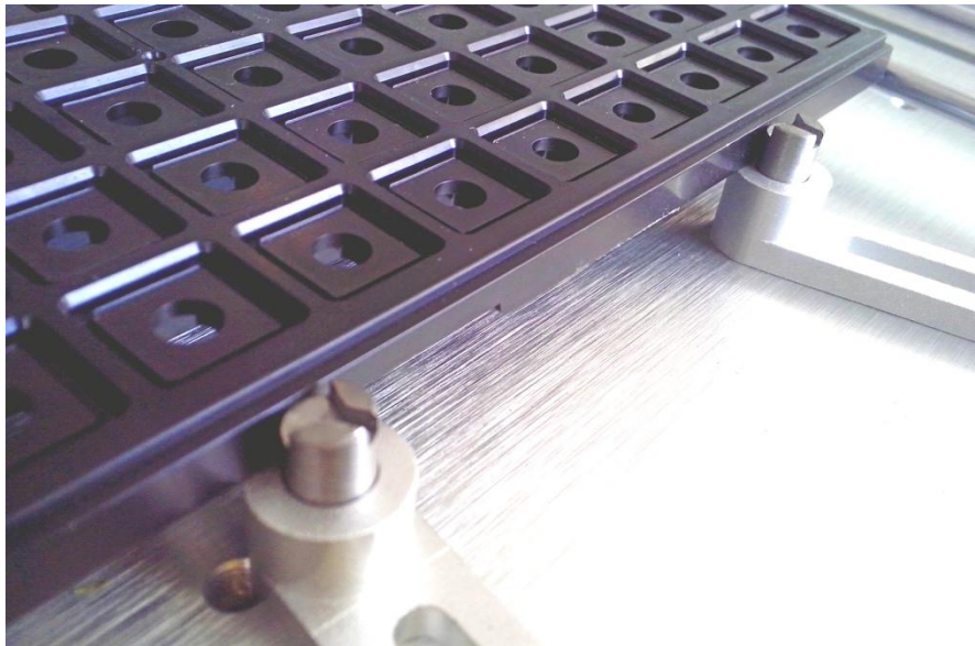
Figure 10.13. Photograph of user IC tray and method for proper clamping.
